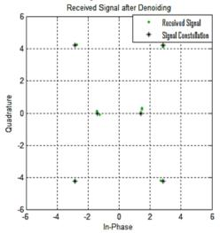
Fig.7. Scatter plot of Denoised signal, Symlets N=1 wavelet Filter
