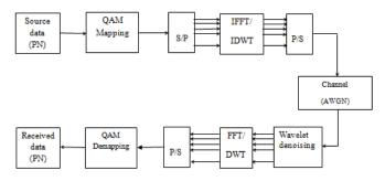
Fig.1 OFDM-DWT Transceiver
