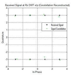
Fig.10. Scatter plot of signal after Wavelet Reconstruction
