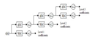
Fig.3 Structure of 3-Level wavelet decomposition
