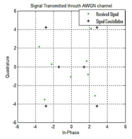
Fig.6. Scatter plot of noisy (AWGN) signalfor SNR=22db and transmitted signal on the same axes.
